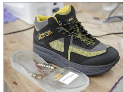
Figure 1 | Shoes that harness the energy generated by footsteps could be used to power mobile devices on the go. (Credit: University of Wisconsin-Madison College Of Engineering.)
