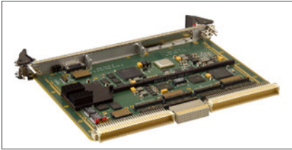
Figure 1 | The VME-194B VME SBC is getting an upgrade from the original Tempe-based design; the board will feature Curtiss-Wright's new FPGA-based VME interface while remaining pin- and feature-compatible with previous generations of VME boards.
